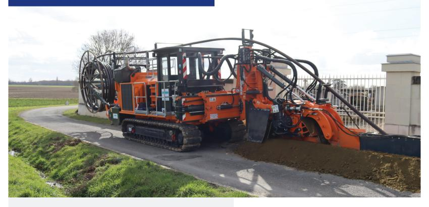
Tesmec ST2 is a 25-27 metric ton-class trencher featuring a 510 HP (375 kW) Tier 4/Stage V engine, or a 536 HP (394 kW) Tier 3 engine, designed to allow the simultaneous trenching and mechanical laying for the deployment of networks in rural environments and rocky grounds
